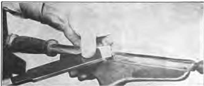
Fig. 183. Turning Wooden Blank for Screw.
